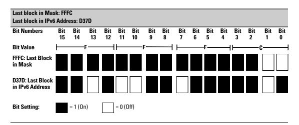
Figure 6-4. Example: How a Mask Determines Four Authorized IPv6 Manager Addresses
